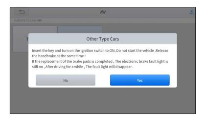
3. Enter the **Enter maintenance mode** menu and release the handbrake brake. And press **OK** after completing the instructions shown.
